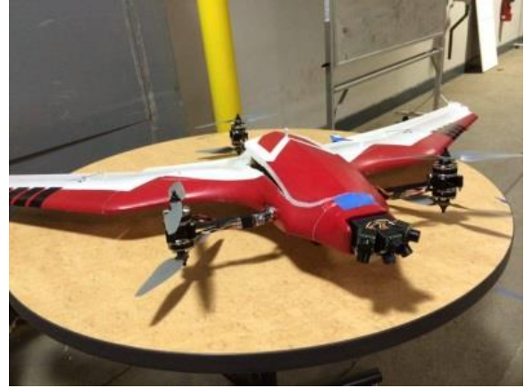
Figure 8: Image Showing 6 Ultrasonic Sensors Mounted at the Nose of the UAV
