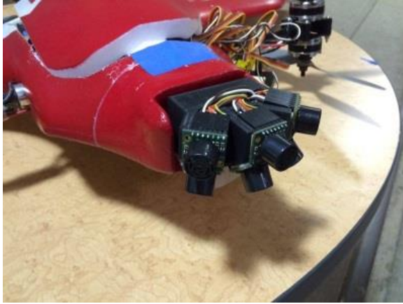
Figure 7: Close Up of 6 Ultrasonic Sensors Mounted at the Nose of UAV
