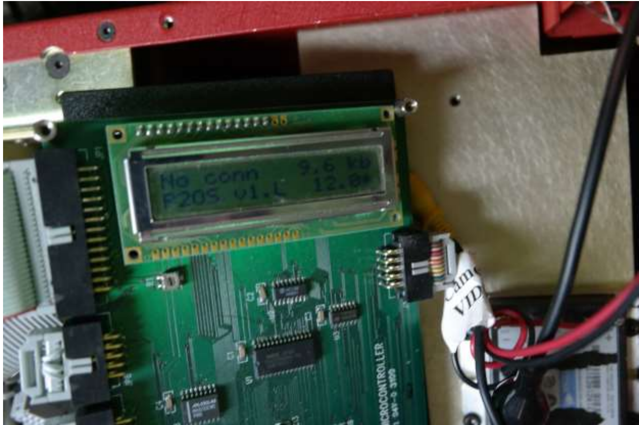
Figure 2: LCD Readout of Pioneer 2
