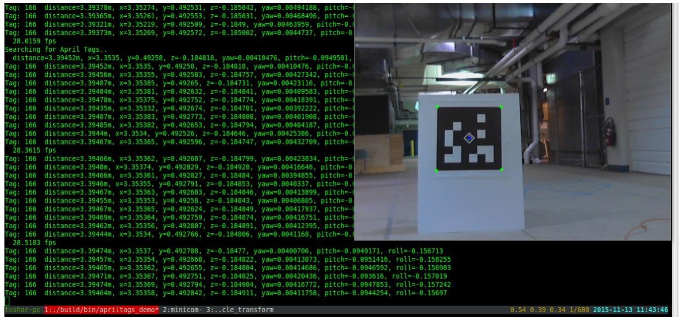
Figure 3. Nested AprilTag outer marker detection. Green Dots indicate corners of marker and blue marks the center. (Marker: Nested Apriltag, Distance: 3.39m, FPS: 28)
