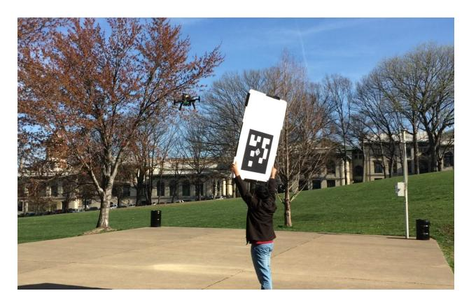
Above shown is a picture of the test where UAV finds an obstacle while doing lawn mover search and tries to avoid it. Testing further the planner failed to produce path at times. In the coming days I will further play around with different planning parameters by looking at the reasons for which parameters cause this problem. This is the final step of the obstacle avoidance subsystem and I will do this in the coming week.
