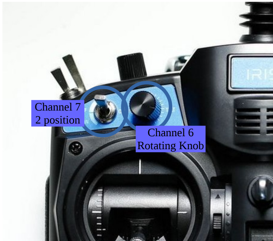
Image 1: The RC controller showing channels 6 and 7. As seen, CH6 can accommodate all PWM values whereas CH7 can only accommodate 2 positions
