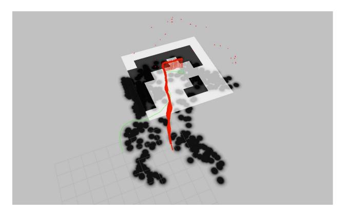
The black spots show the obstacles as registered by the costmap. The red dots are lidar value when there is no obstacle in front of it. The green path is the path generated by the navigation stack.
