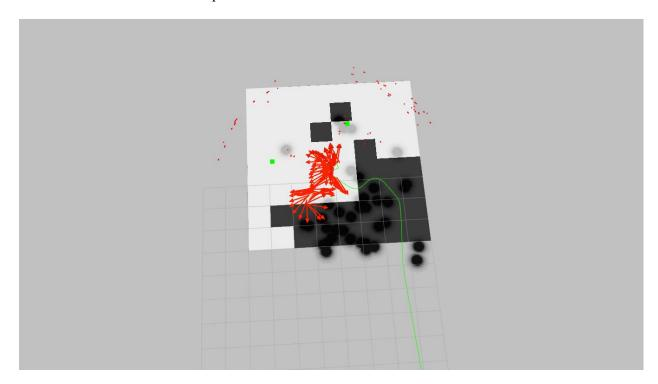
In the above figure the red spots are unfiltered output from our previous indoor sensor. The 2 green dots are the filtered output. As seen the noise is greatly reduced by median filter.
