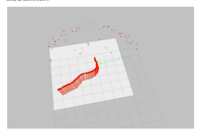
As a result of the above shown noisy data the costmap though there are many obstacles around the UAV and so the navigation stack generated a path avoiding all those obstacles which resulted to the issue of UAV rotating arbitrary or the planner failing to produce path considering there are obstacles all around the UAV.
