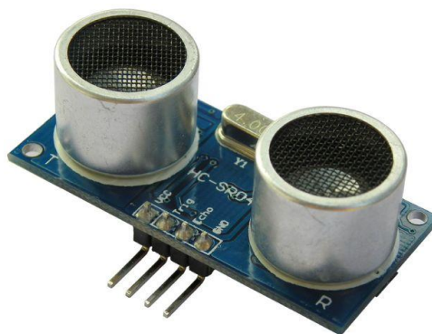
Figure 3: HC-SR04 Ultrasonic Range Finder Sensor (Image Courtesy: Sparkfun.com)
