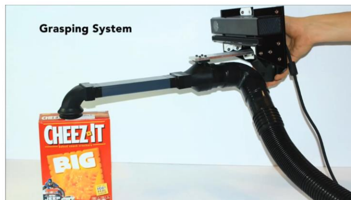
Figure 12: Custom Suction End Effector
