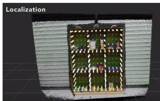
Figure 6: Localizing the Shelf (White Point Cloud) to the Kinect Image
