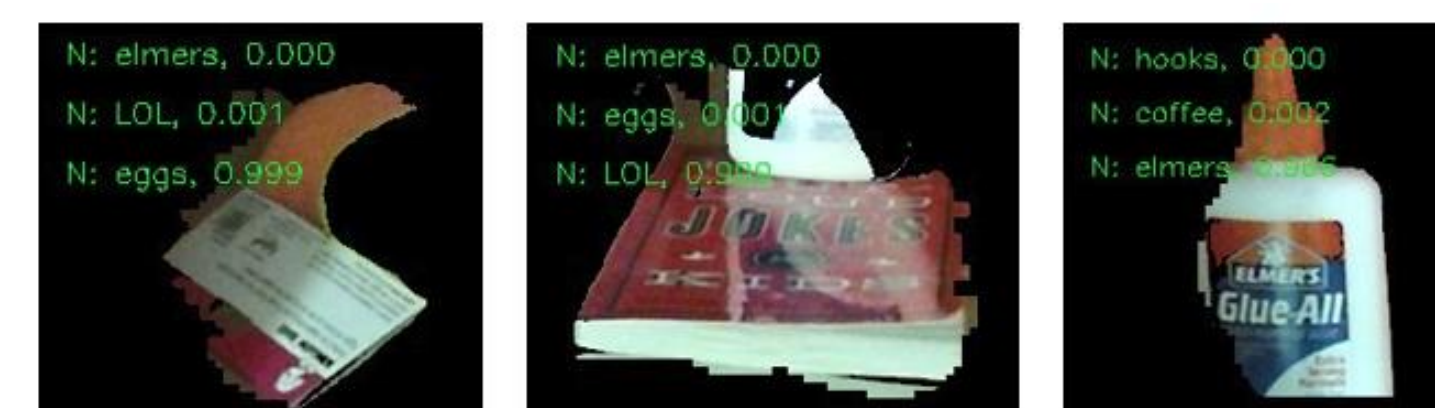
Segment Identification: Individual segments are classified using a CNN
