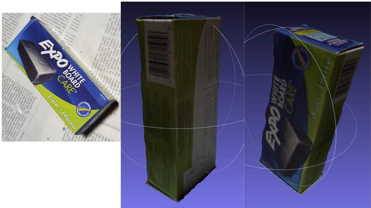
Figure 2: Generated 3D model white board eraser
