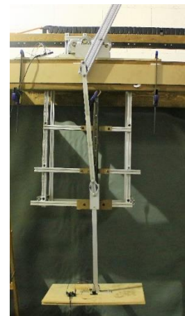
Figure 14: Crank Slider mechanism of Docking Platform
