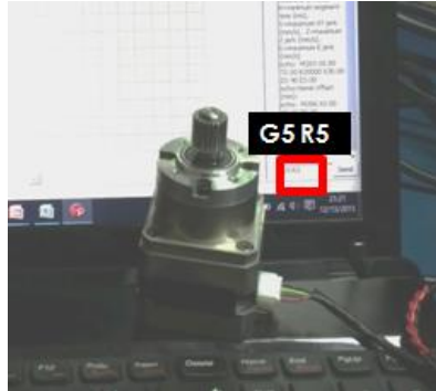
Figure 21: R-axis stepper motor controlled using G5 command from the pronterface software
