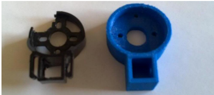
Figure 2: Example of failed 3D printed motor mount and a less desirable ‘thickened’ replacement necessary to support the loads. ( http://www.wattflyer.com )
