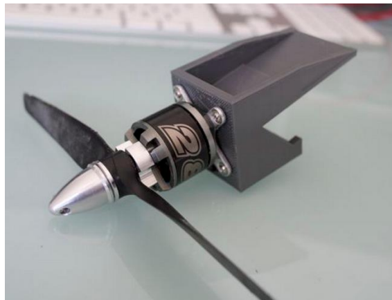
Figure 5: Motor mount made with ADD_IN printer ( http://www.anzel360.com/category/rc/fixed-wing/ )
