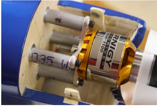
Figure 4: Time intensive aluminum and balsa motor mount. ( http://www.rcgroups.com )
