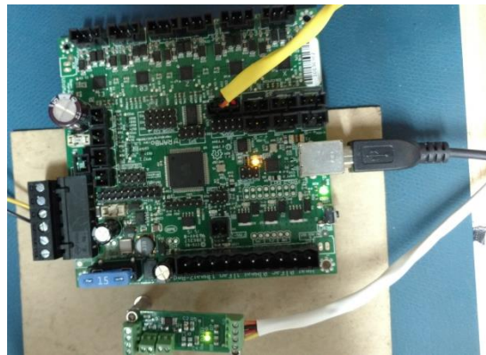
Figure 22: Custom PCB and RAMBo board under testing
