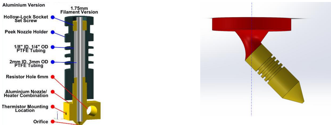
Figure 7.4: View of standard 3D print nozzle (left) and rendering of inclined nozzle concept for 4DOF
