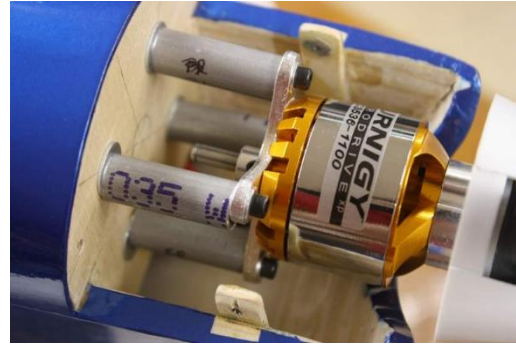
Figure 2.4: Time intensive aluminum and balsa motor mount. ( http://www.rcgroups.com )
