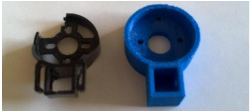
Figure 2.2 Example of failed 3D printed motor mount and a less desirable ‘thickened’ replacement necessary to support the loads. ( http://www.wattflyer.com )
