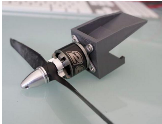
Figure 2.5: A 3D printed motor mount with internal stiffeners and screw inserts printed by 4DOF
