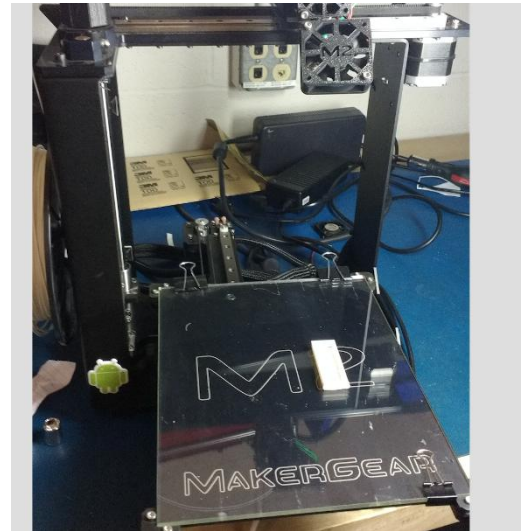
Figure 2.12: Printer in insertion configuration awaiting COTS item installation
