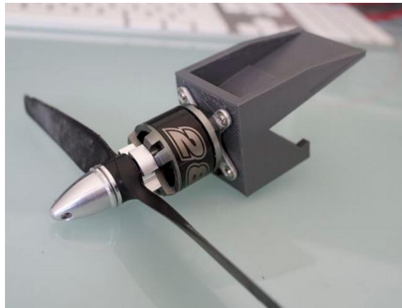
Figure 5: Motor mount made with ADD_IN printer ( http://www.anzel360.com/category/rc/fixe-wing/ )
