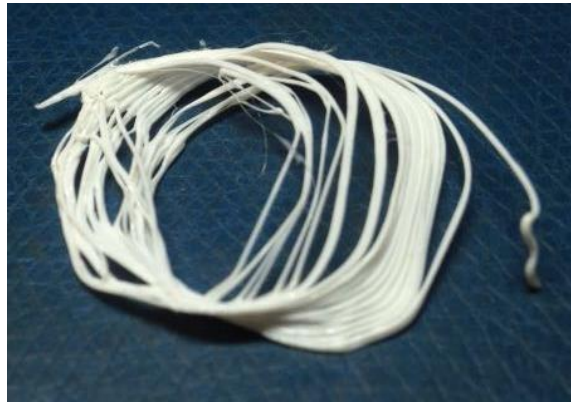
(c) Drift seen while printing a thin cylinder
