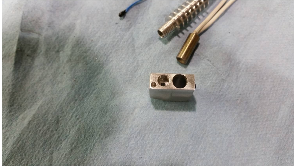
Figure 1: Custom heat block + barrel after manufacture prior to assembly. The constriction is visible through tapped hole on left of image.
