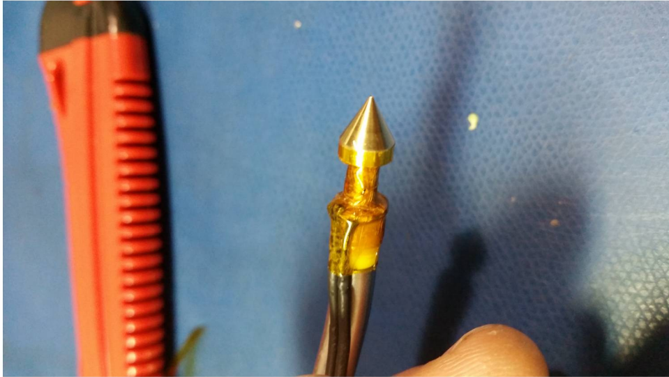
Figure 3: New nozzle design prior to winding of the heating coil. A used thermistor is installed which will eventually failed from handling.
