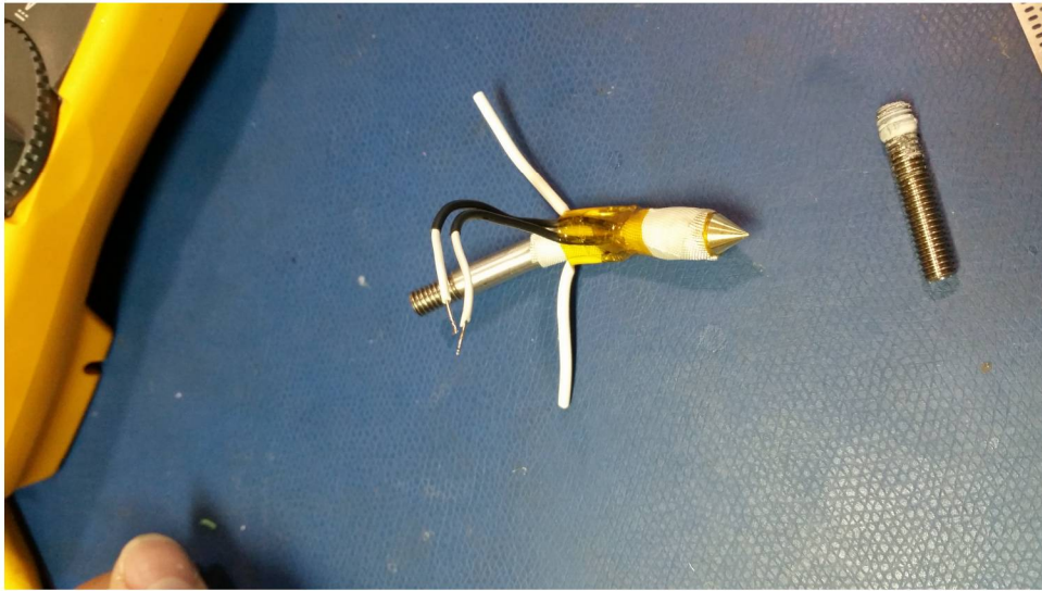
Figure 4: New nozzle design with heating coil completed.
