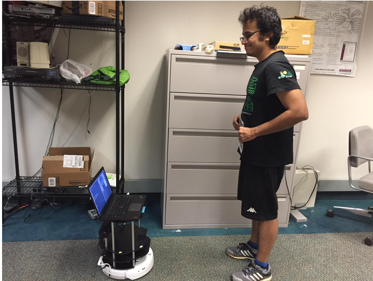
Turtlebot detects april tag, navigates and stops at a distance of 100cm from the detected human
