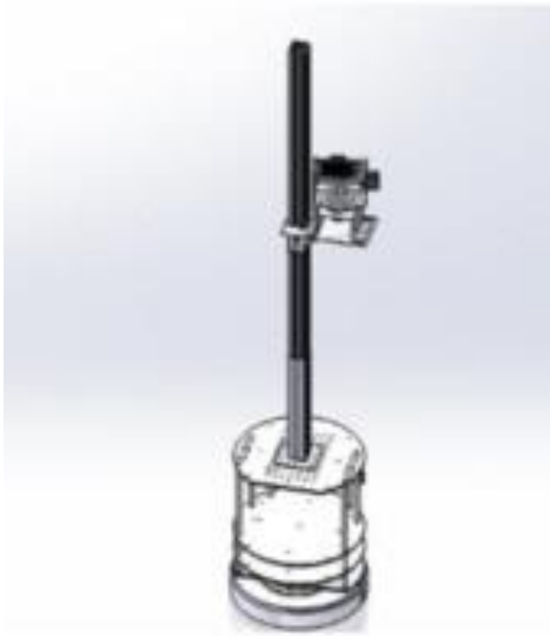
Figure 8 CAD model of Pan-tilt +Elevation rod unit mounted on turtle bot
