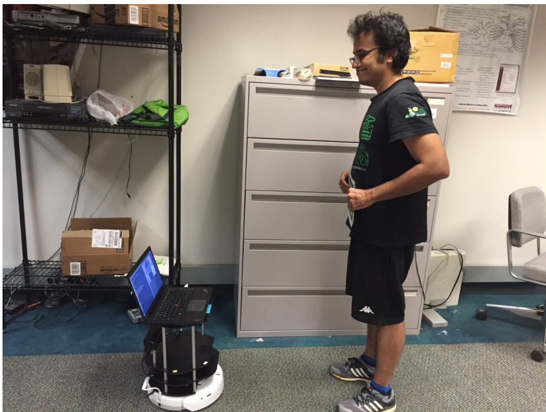
Figure 13 Turtlebot successfully detects the human and navigates towards it. Stops at 100 cm away from the human.
