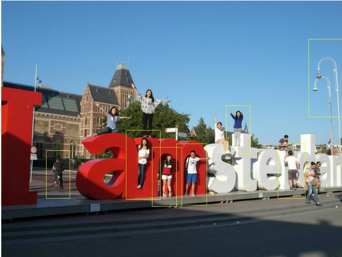
Drawing 1: The result of human detection using HOG algorithm
