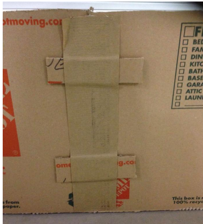
Figure 12: Reinforced Joints in Cardboard Mock Parking Lot
