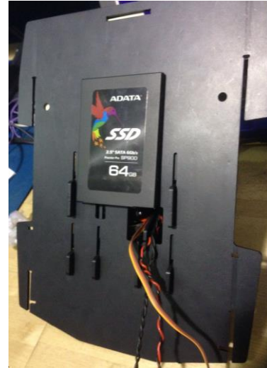
Figure 6: SSD Card on Bottom of Upper Assembly
