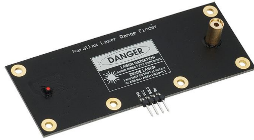
Figure 2: Parallax Laser Range Finder, www.robotshop.com
