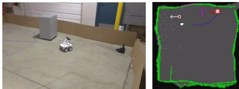
Figure 2: Blue path shows the trajectory calculated to avoid the obstacle
