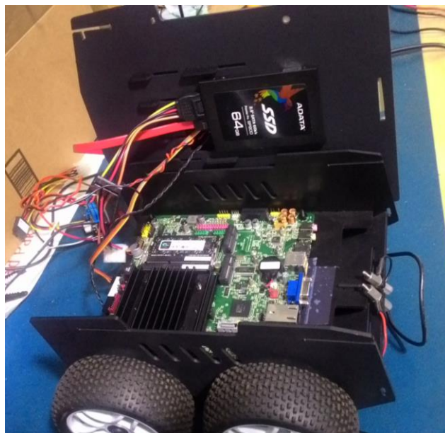
Figure 2. Platform interior with Intel DN2800MT and SSD
