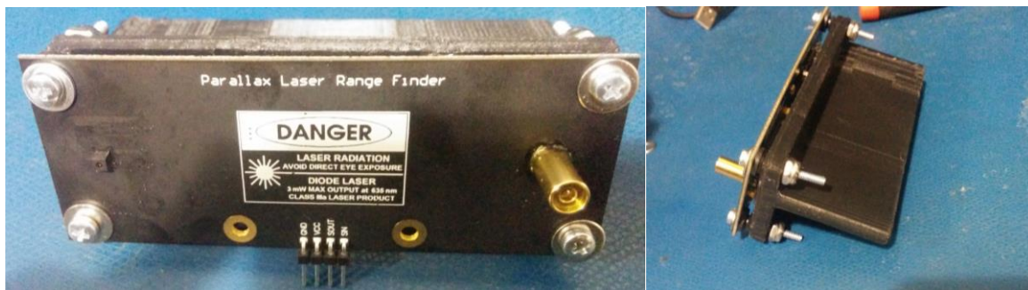
Figure 5- 3D printed mount with sensor
