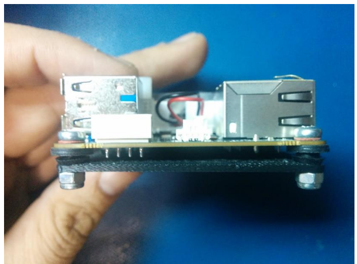
Figure 6- 3D Printed base plate for SBC
