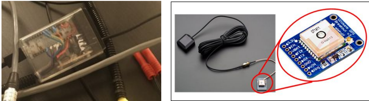
Fig. 10. (Left) The Arduino Module box includes a 12 VDC voltage regulator and an Arduino Micro. The plug on the left connects to the camera GPIO pins; the one on the right is an HXT connector for the battery. (Right) The Adafruit Ultimate GPS sensor and its antenna are designed to work with Arduino boards.
