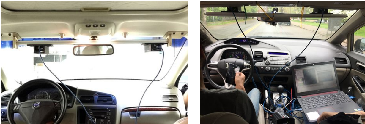
Fig. 9. The vision subsystem consists of the cameras and their mounting solution
