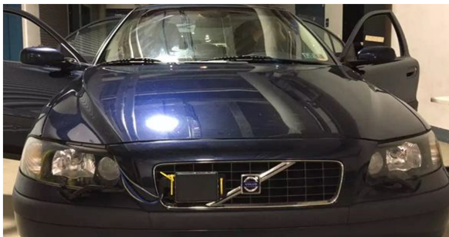
Fig. 12. The radar is mounted on the grille, while the stereo-vision setup is installed inside the car cabin.
