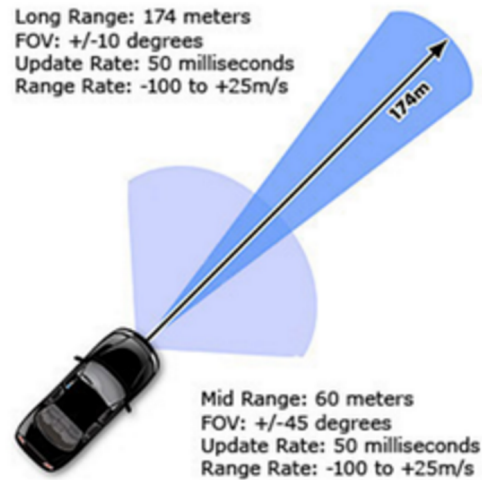
Figure 4. Radar Range Representation
