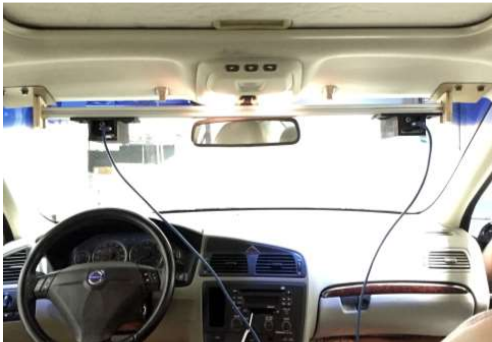
Figure 1. On-board setup of the cameras
