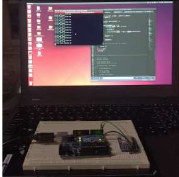
Figure 3. Outdoor Testing of the GPS module
