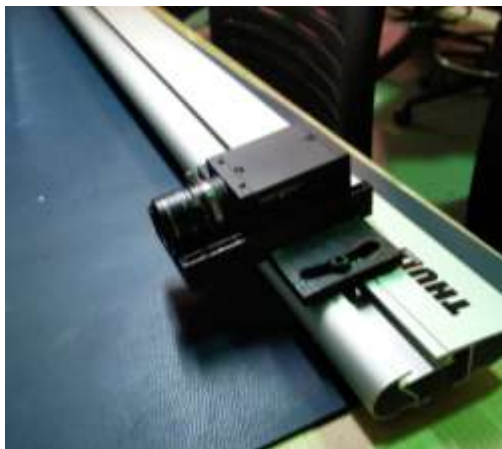
Figure 2. 3D-printed prototype of the camera housing
