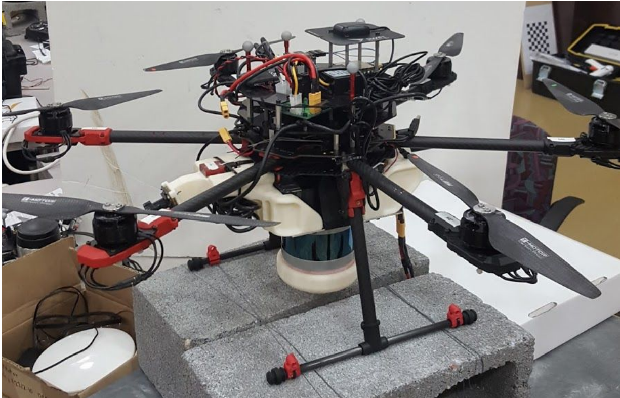
Figure 10: UAV with all sensors and hardware mounted
