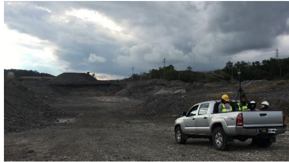
Figure 9: Bagging data at the Lafarge quarry with the Velodyne Puck Lite and Piksi GPS.
