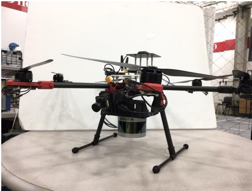
Figure 3: Hexrotor vehicle with GPS, IMU, RGB Camera, LiDAR, battery mounted
