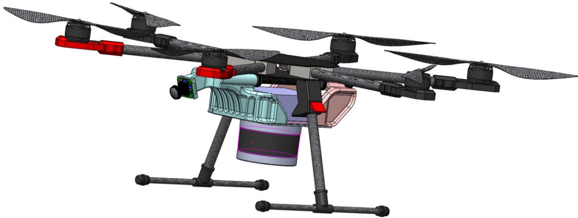
Figure 2: CAD of hexrotor vehicle with sensor mounts
