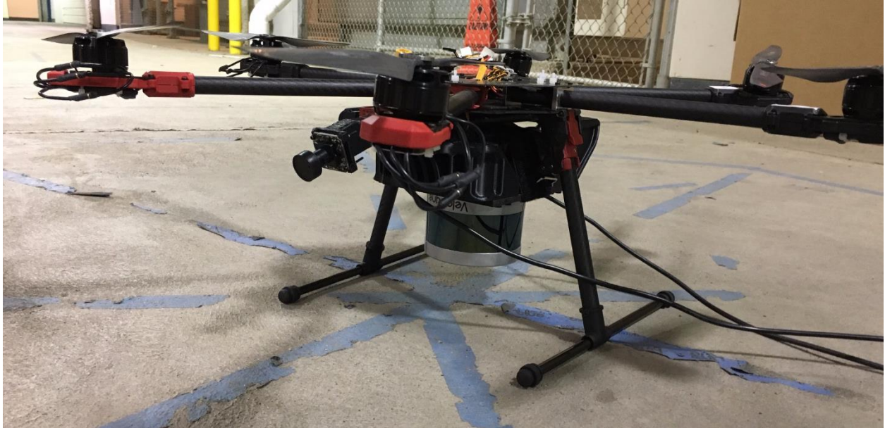
Figure 5: Physical UAV with 3D printed sensor rig mounted.
