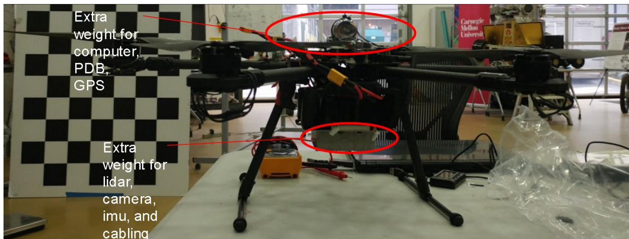
Figure 2: UAV with dummy payloads attached. Credit to Angad Sidhu for the image and labeling.
