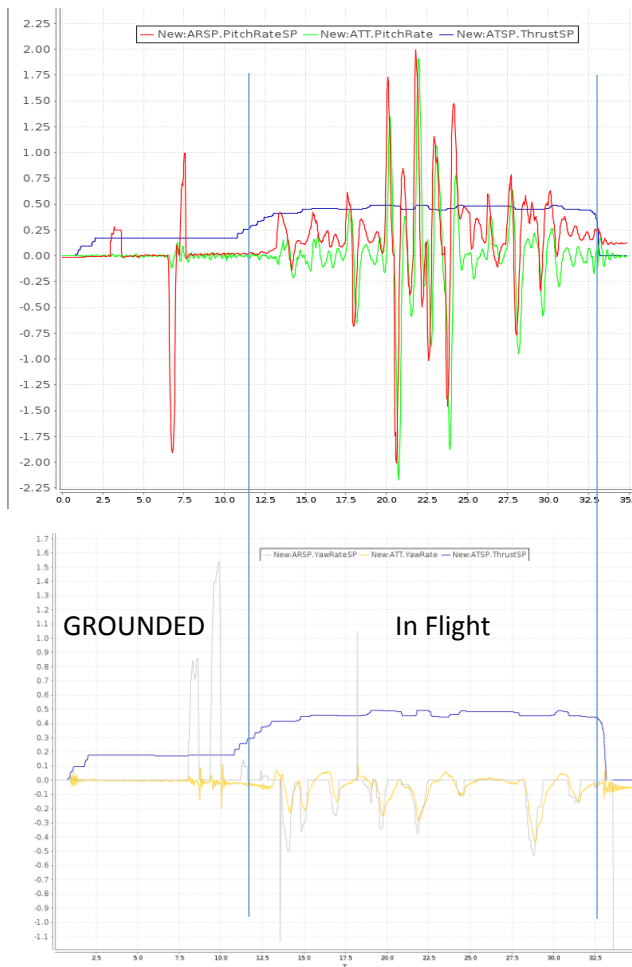
Figure 1: Flight Plots with the blue curve in both denoting the thrust, and appropriate flight state demarcated as “Grounded” or “In Flight”. Top – Plot of pitch rate with set point in Red and measured values in green. Bottom – Plot of Yaw rate with set point in Gray and measured values in Yellow.
