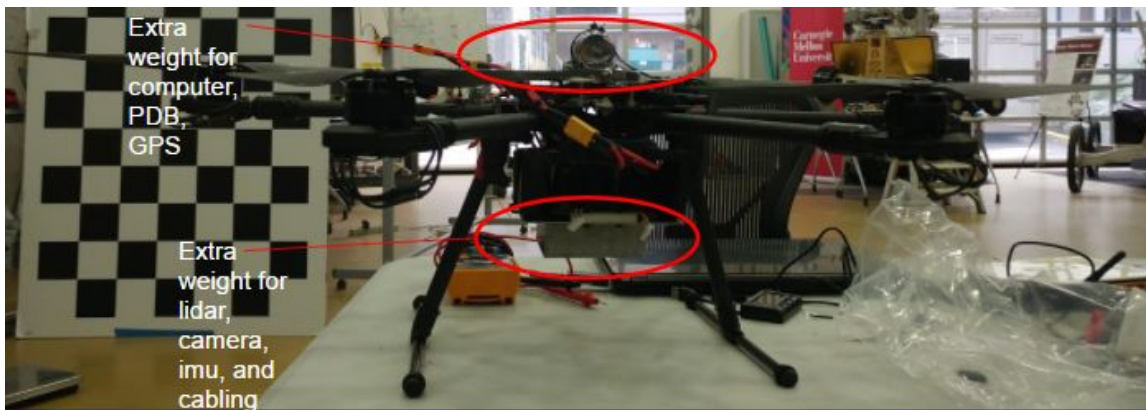
Figure 17: Shows test setup for dummy payload test.
