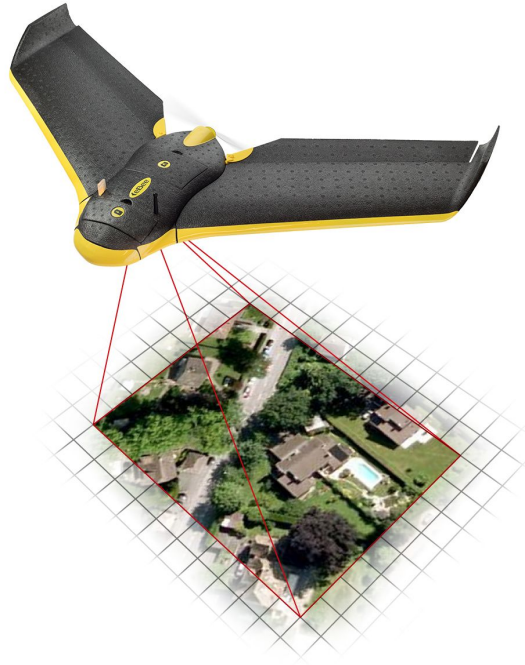
Figure 5: Sensefly fixed-wing surveying UAV
