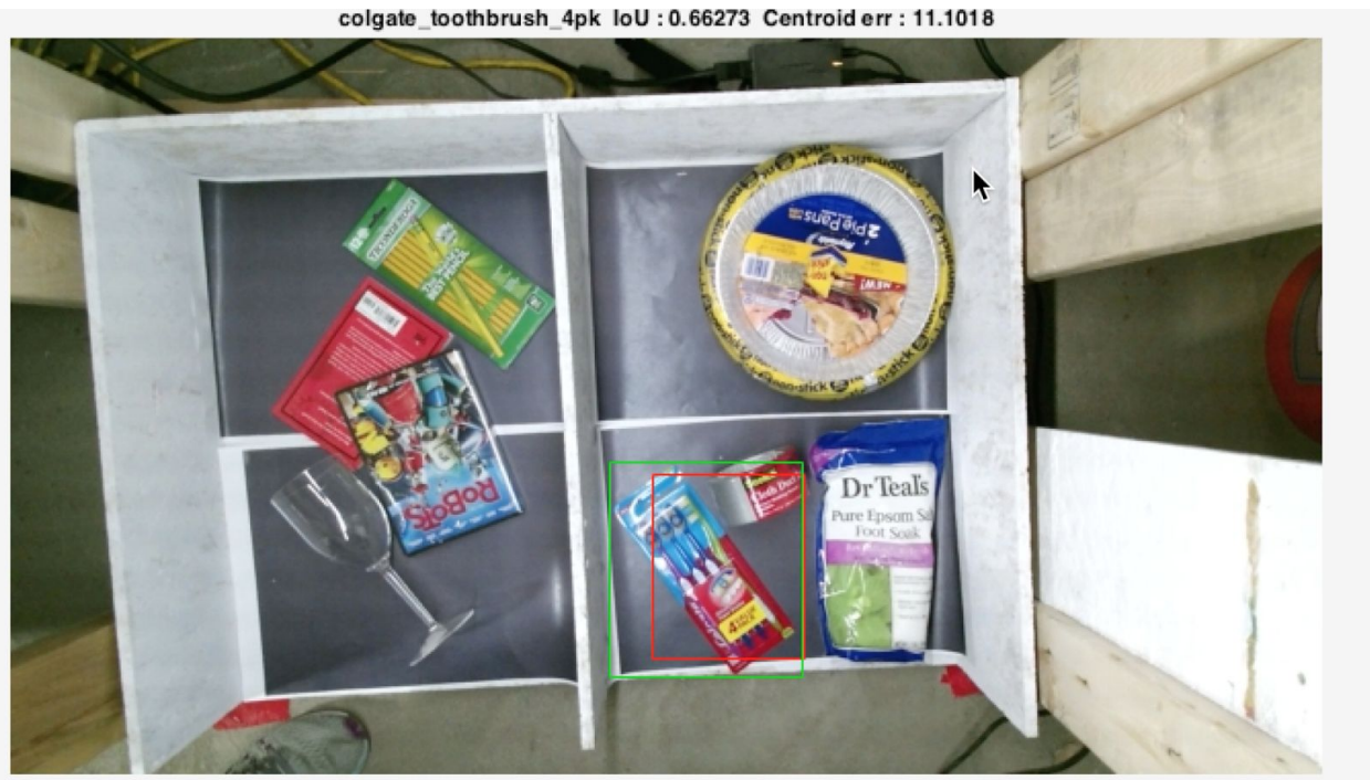
Figure 2. Faster RCNN prediction using testing set
