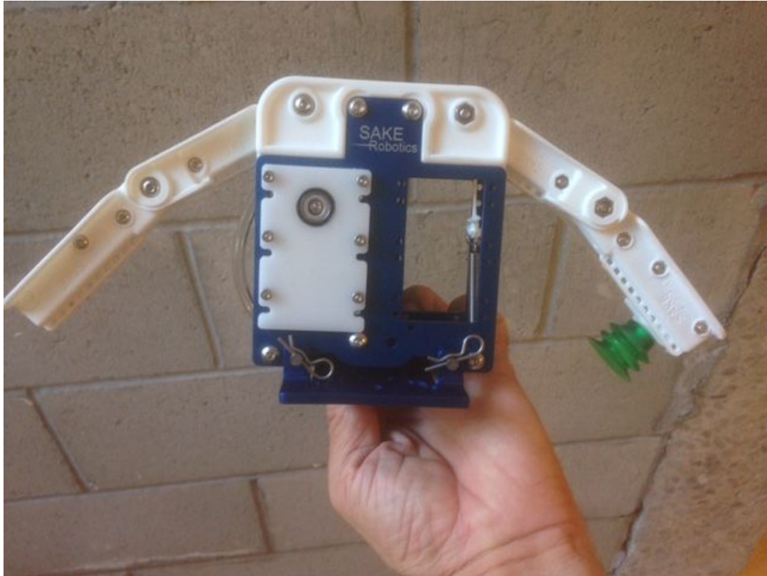
Figure 3. SAKE Robotics two-finger gripper. The suction cup is a Piab bx25p and is an optional attachment.
