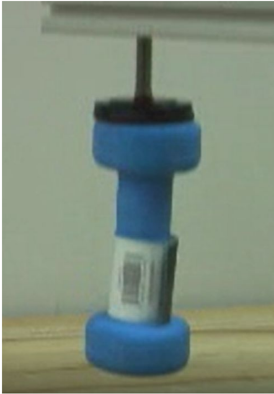
Figure 4. Anver suction systems for lifting the dumbbell (left) and package of Oreo's (right).
