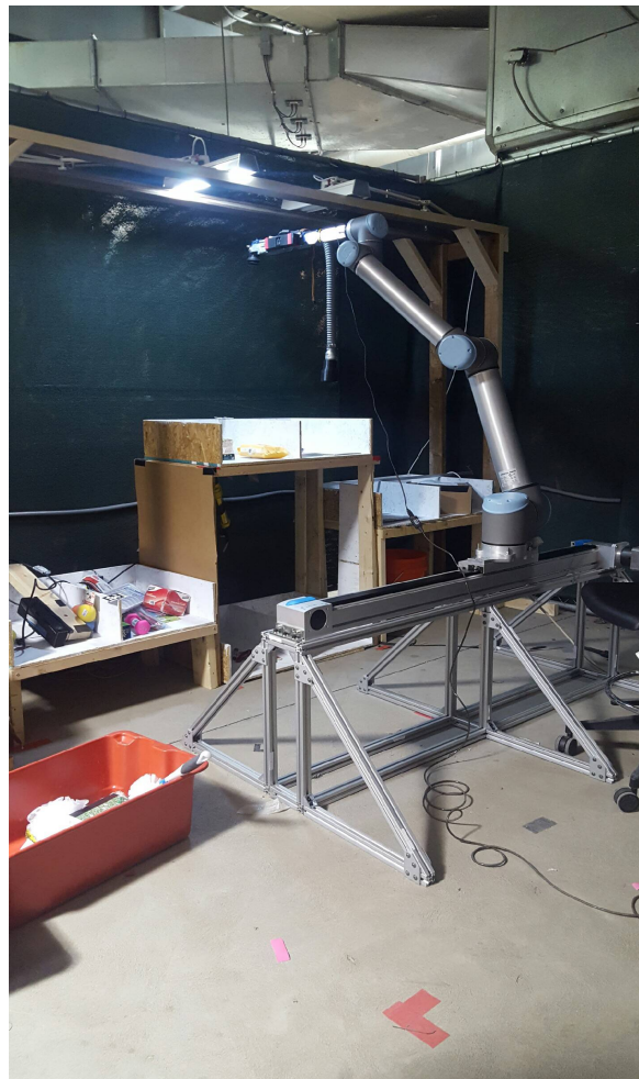
Figure 3: Our project arm mounted on the new 80/20 stand. The stand provides the necessary reach to all system bins.
