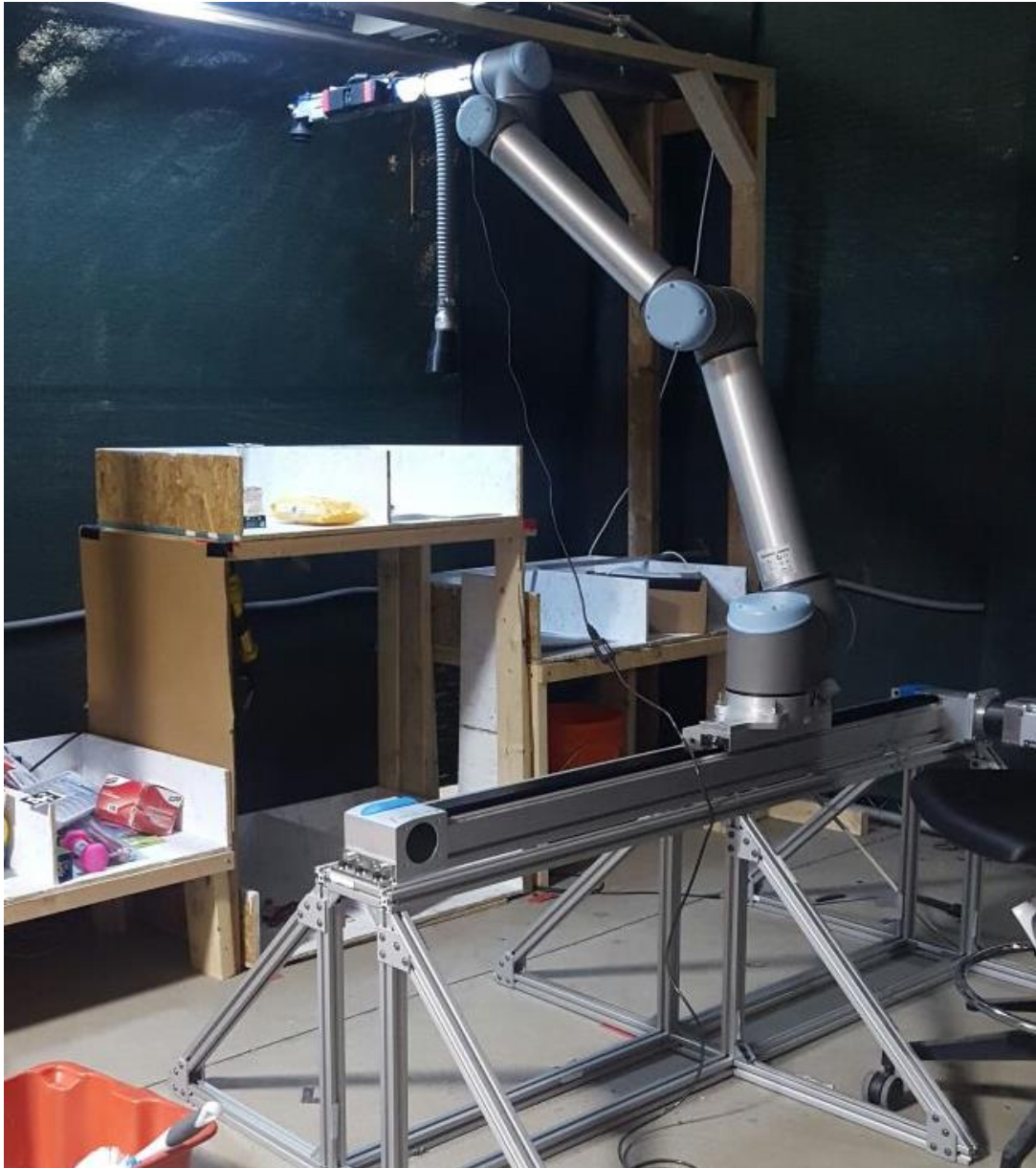
Figure 2. The arm taking an image of items during a partial test run.
