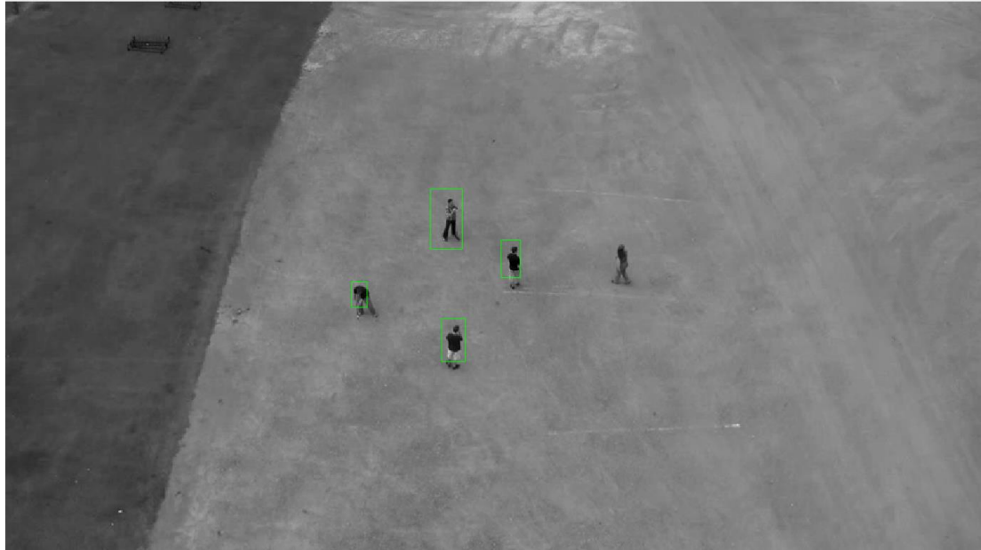
Figure4 Result of blob detection method
