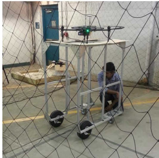
Figure 3: Sound sample collection: The propellers were running and being given thrust through RC. I and Karthik were shouting in close vicinity. Mobile phone to record the sound was kept on the ground.
