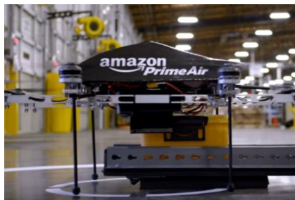
Figure 1: Amazon Prime Air: Design 1: Two clasps on the drone, designed specifically to lock on specially-designed boxes
