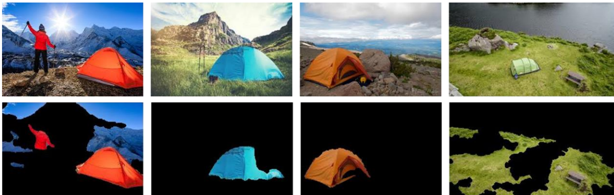
Figure 1: Extraction of bright regions from images using 'HSV thresholding'. The algorithm seems to work fine for most of the cases but loses its purpose when the object of interest is dull (illustrated in the right-most set)
