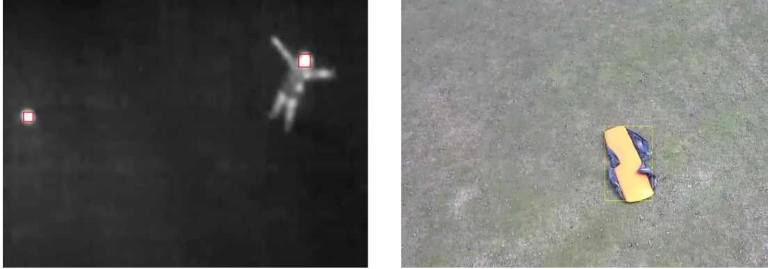
Figure 2: (a) Hot object detection using intensity thresholding in thermal images, (b) Bright-colored object detection using HSV-thresholding
