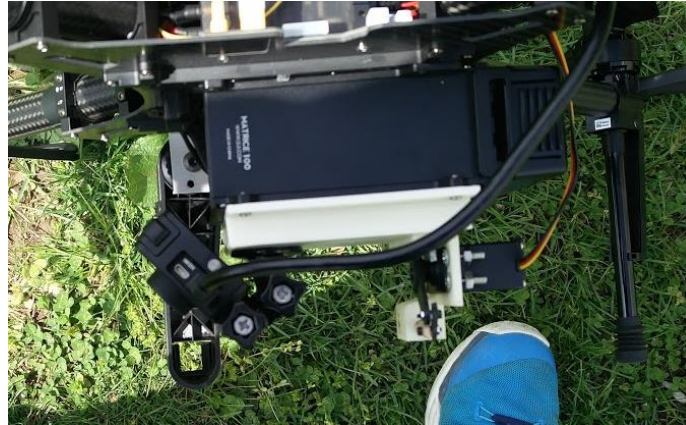
Figure 4: Camera and package drop mechanism mounted on the drone together
