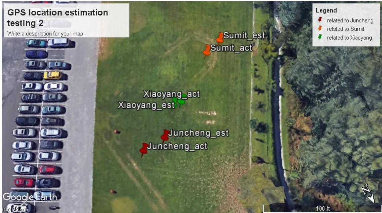
Figure 3: Google Earth plot showing locations of all the signatures – both actual and estimated (second round of testing)
