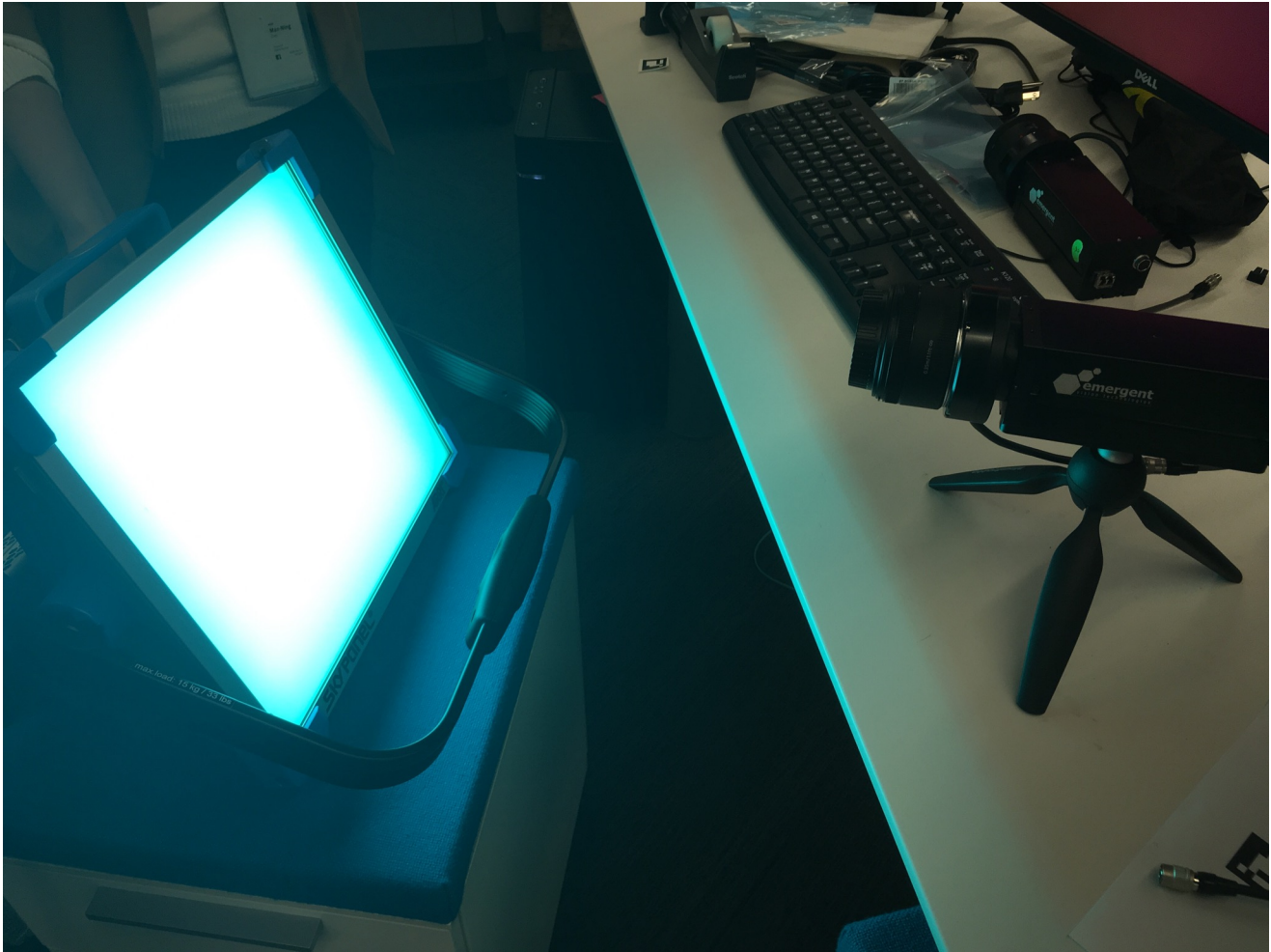
Figure 4. The uniform light source and the EVT 12000 camera
