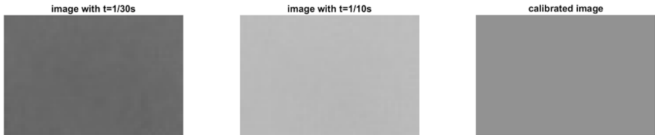
Figure 2 -1. The result of implementing CRF algorithm (at least two images with different exposure time is needed, and more images will produce more accurate results)
